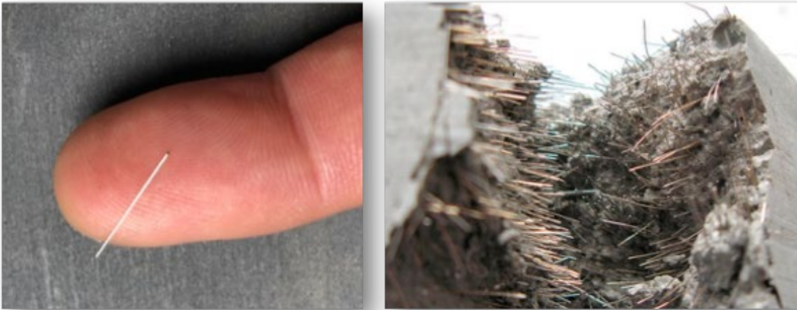
FIGURE 2: Steel fibers are a critical component of UHPC
