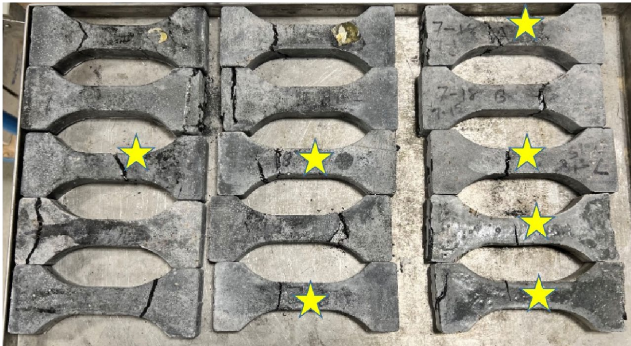
FIGURE 21: Field cast tensile coupons. Curves in Figure 21 are from specimens marked with a star, which are ones that failed in the gage length. NOTE: Specimens were made by field staff with no experience in collecting tensile samples
