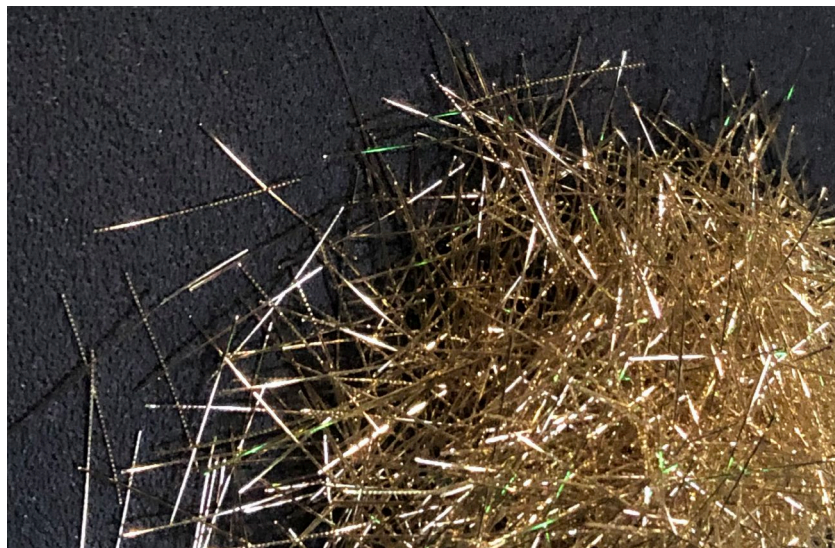
Striated Type X fiber developed in this project. Light reflection from the surface striations can be seen on the fibers.
