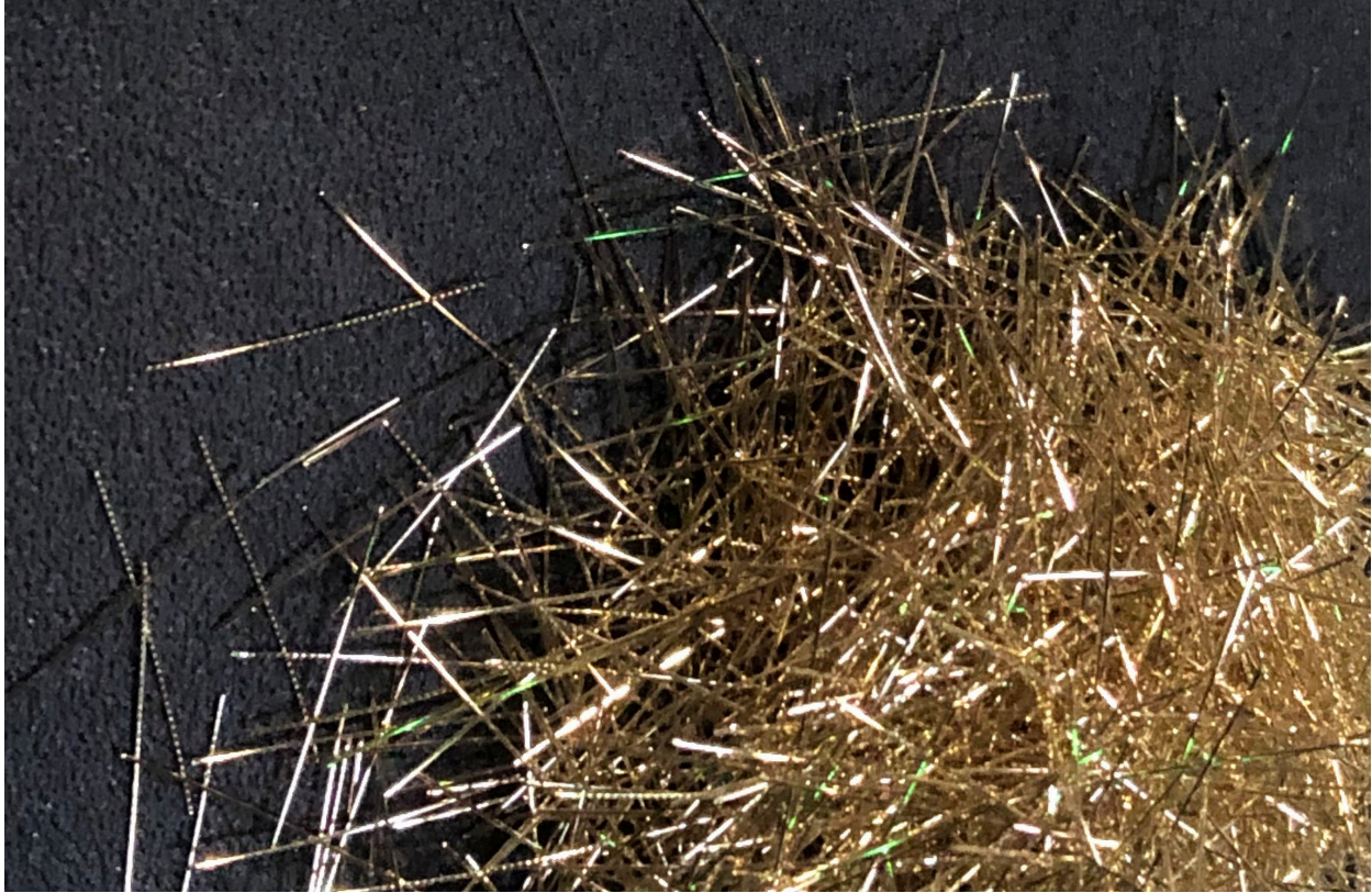
FIGURE 5: Fiber production sample from new machine (new Type X fiber). Light reflection from the surface striations can be seen on the fibers
