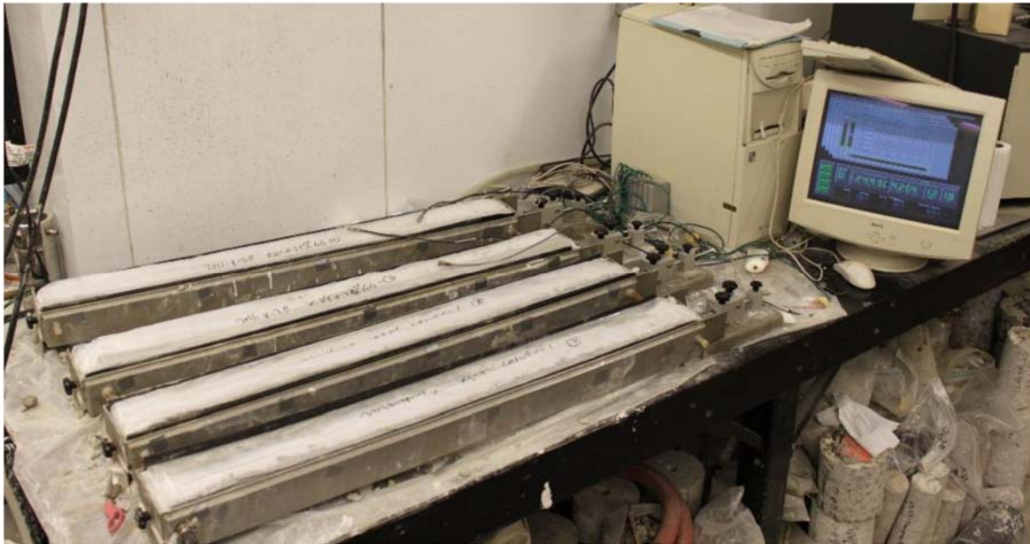
Figure 4-2 Autogenous shrinkage measurement
